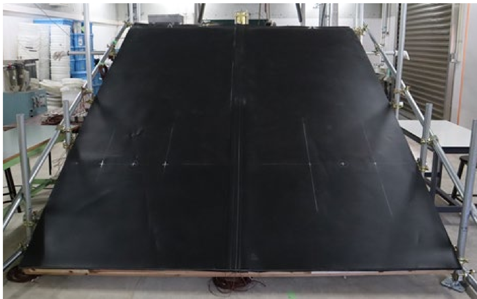
Slope Model with Impermeable Liner Laid
