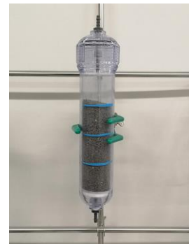
Photo3 Incinerator ash packed column
